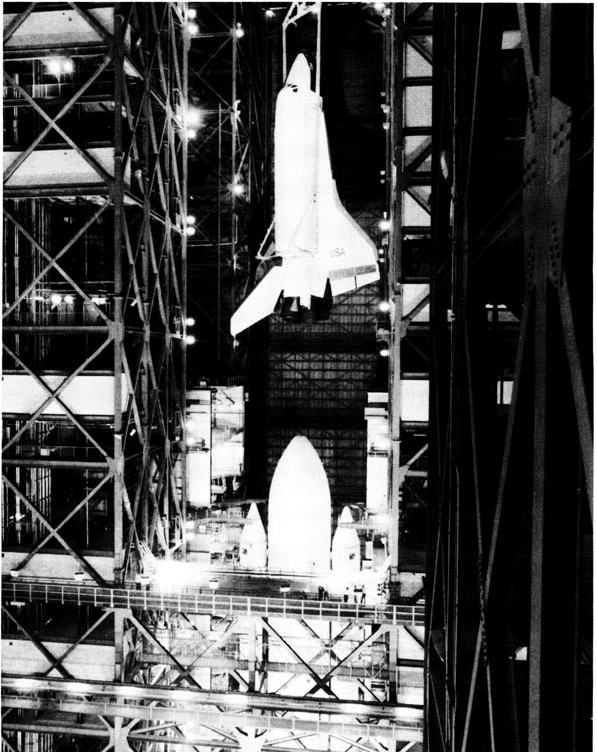
FIGURE 15 – ORBITER MATING WITH EXTERNAL TANK AND SOLID ROCKET BOOSTERS
